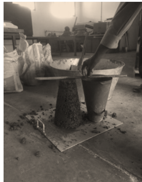
Fig. 6. Slump test in progress
